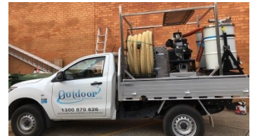
Water extraction system on a removable skid
