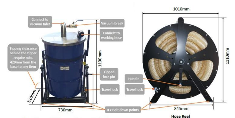
Drum Tipper with Drum and interceptor head
